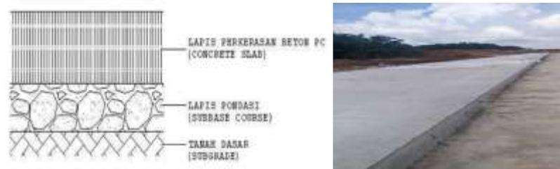
Gambar 2. 1: Perkerasan Rigid
