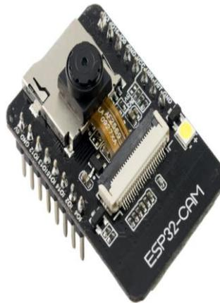
Gambar 2. 1 ESP32-CAM
