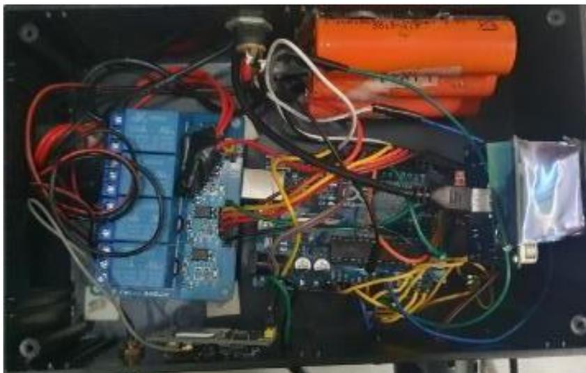
Gambar 3.5. Bagian Kontrol Alat Monitoring Banjir
