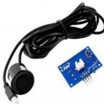
Gambar 2.8. Sensor ultrasonik JSN-SR04T (Ardhiya, 2021)
