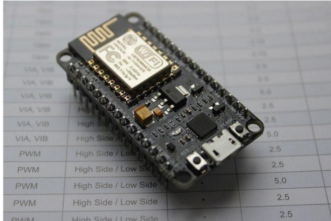
Gambar 2.2 NodeMCU V2
