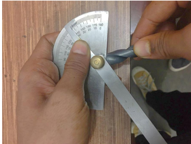
Gambar 4.4 Proses mengukur sudut twist drill
