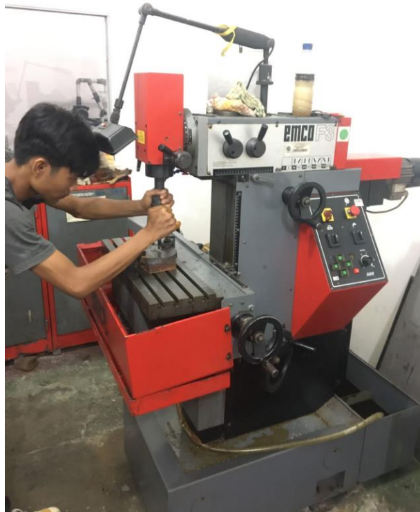
Gambar 4.1 set up mesin NC mill F4
