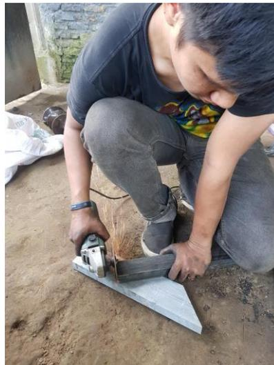
Gambar 4.2 Memotong Besi UMP
