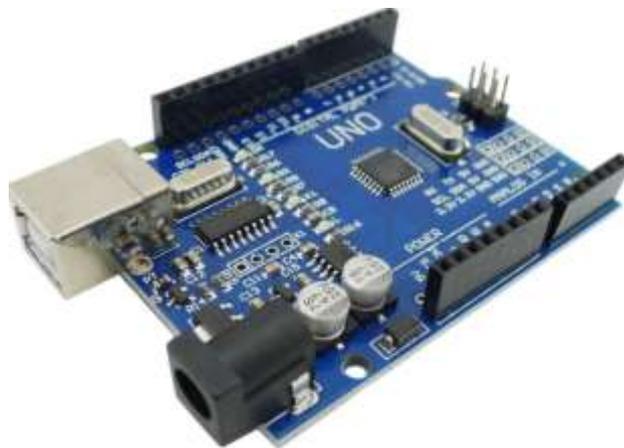
Gambar 2.2 Mikrokontroller Arduino Uno
