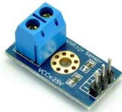
Gambar 2.6 Voltage Sensor
