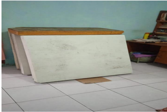
Gambar 3.1 Panel Cold Room
