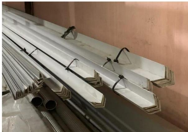
Gambar 3.8. siku alumunium
