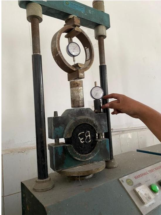
Gambar L.17: Proses *Marshall Compression*
