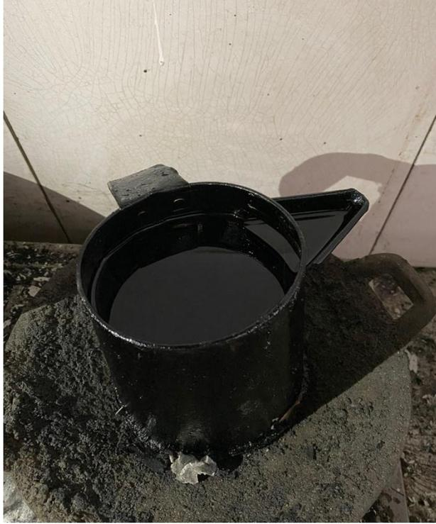
Gambar L.3: Aspal Penetrasi 60/70
