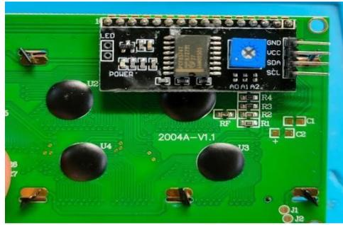
Gambar 3.8. Modul inter integrated circuit
