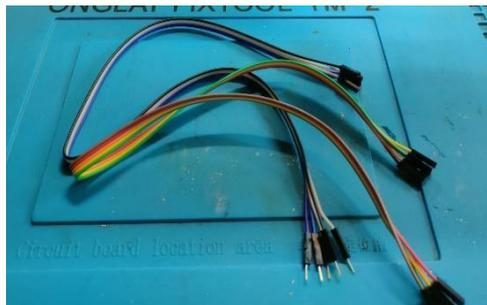
Gambar 3.7. kabel jumper female-male
