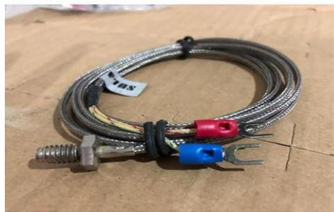
Gambar 3.5. Sensor suhu termokopel type-K
