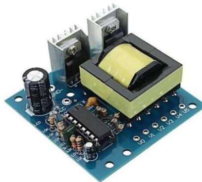
Gambar 3.14. PSU 220v AC-36v DC
