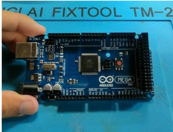
Gambar 3.2. Arduino Mega 2560
