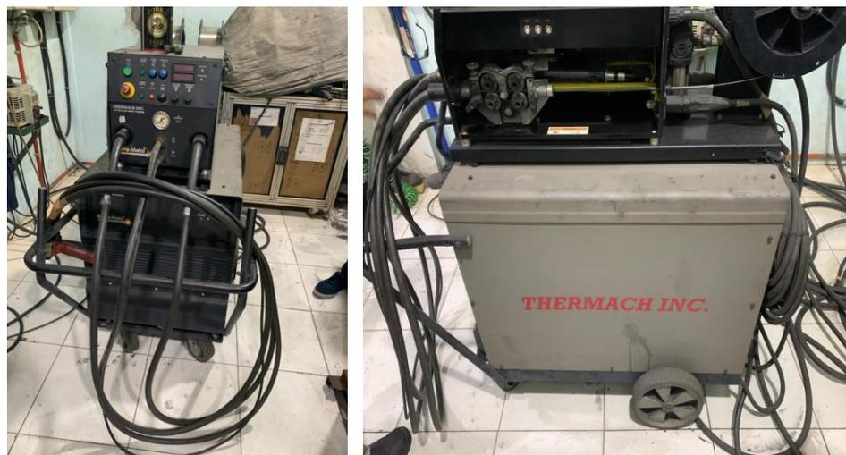
Gambar 4.4 Mesin Metal Spray.
