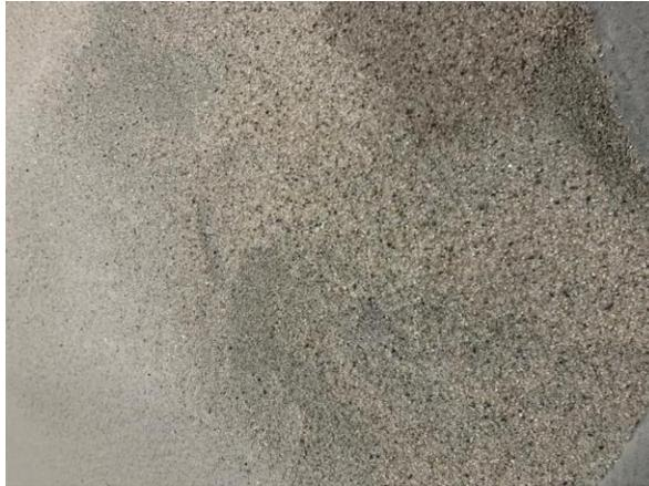
Gambar 4.6 Pasir Aluminium Oxide.
