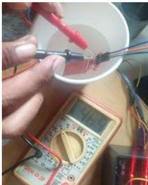
Gambar 4.11 Pengukuran Sensor Water Level
