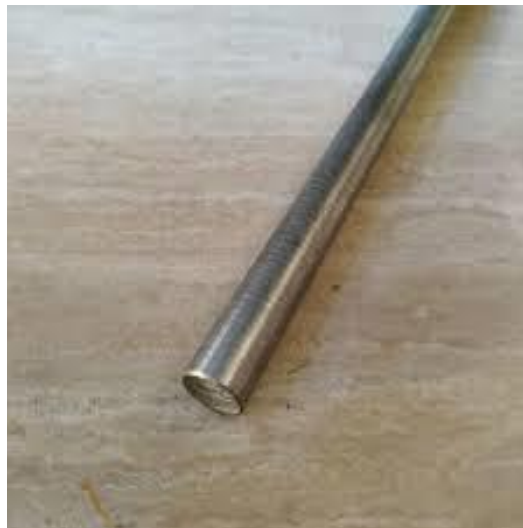
Gambar 4.7 Besi as berdiameter 25,4mm
