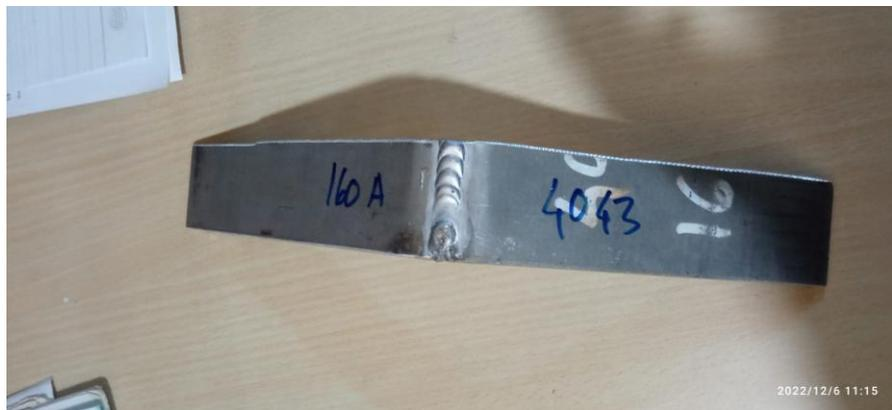
Gambar 4.6. Bending Material hasil *Welded* Spesimen 2
