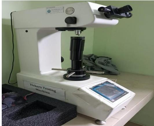
Gambar 2.22 Alat uji kekerasan Vickers Testing Machine (Lab ATB Polmed)
