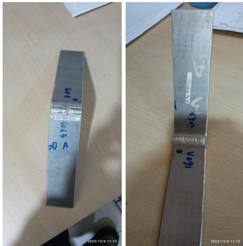
Gambar 4.5. Bending Material hasil *Welded* Spesimen 1
