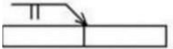
Gambar 2.3. Kumpuh I square butt weld (Aji, 2019)
