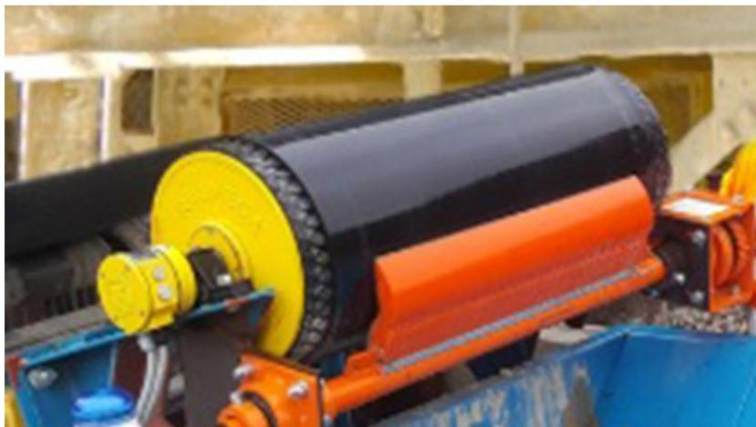
Gambar 2.16. *Belt cleaner conveyor* Otomatis
