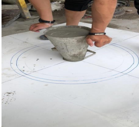
Gambar 2.8 Uji Slump Flow
