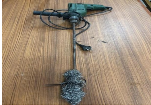
Gambar 3.19 Mesin pengaduk foam agent (bor)
