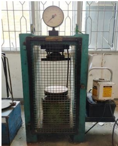
Lampiran 8 : Compressing Test Machine (CTM).
