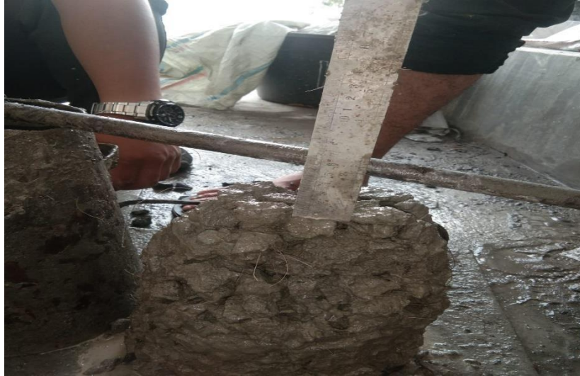
Lampiran 29 : Proses Pengujian Slump Test.
