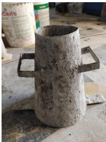
Lampiran 15 : Kerucut Abrams.
