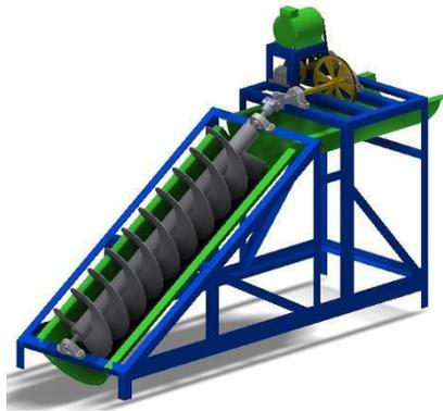
Gambar 2.7 Turbin Screw Archimedes (Muhammad Rifky, 2020)
