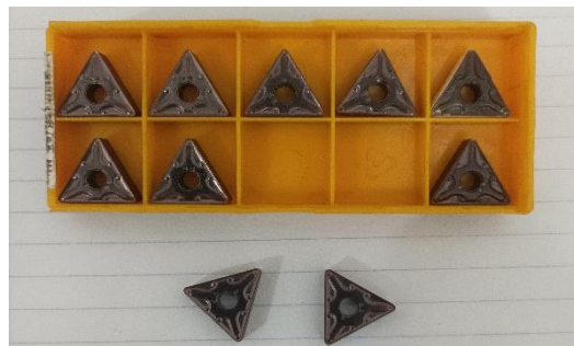
Gambar 3.3 Mata pahat Triangle Insert Turning Type T
