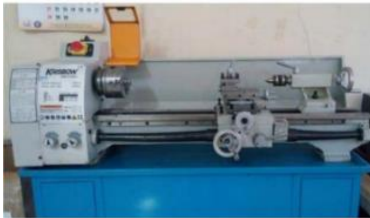
Gambar 2.1 Mesin bubut centre lathe (Sulistyarini et al., 2018)
