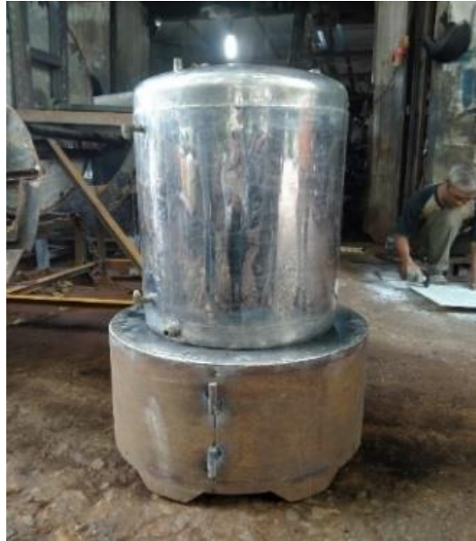
Gambar : 2.9 Badan boiler
