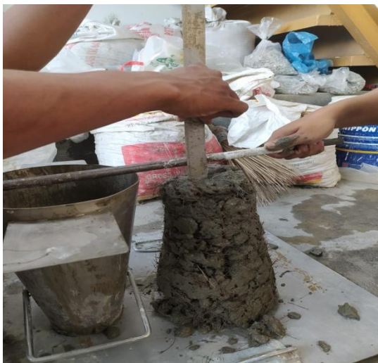
Gambar L-24: Proses pengujian slump test .
