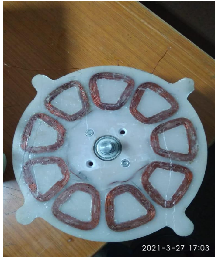
Gambar Stator Generator Axial Flux Magnet Permanet
