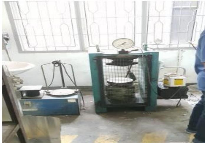
Gambar L.1: *Compressing test machine.*
