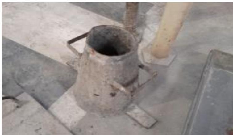
Gambar L.6: Kerucut abrams
