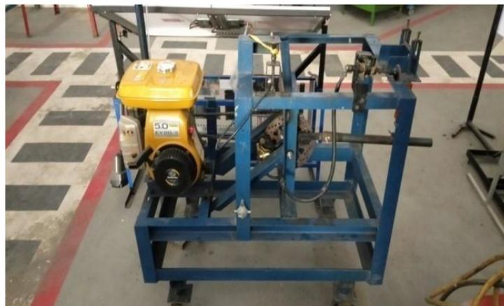
Gambar 3.5 Brake Dynamometer
