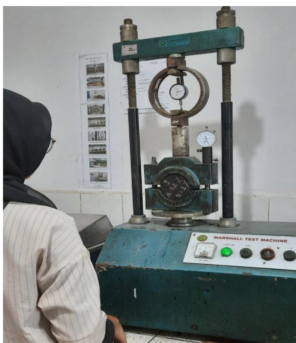
Gambar L12: Proses pengujian Marshall
