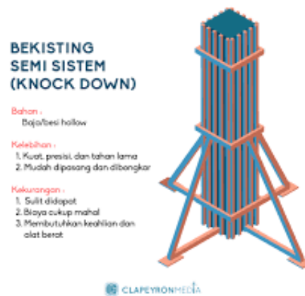
Gambar 2.2: Bekisting Semi Sistem (Hanna, 1999).
