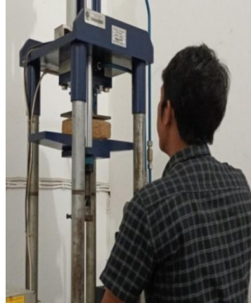
Gambar -16 Alat Uji Kuat Tekan (Compression Test)
