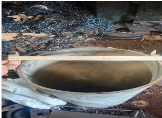
Gambar 3. 5 Besi Tabung ukuran diameter 210 mm x 5 mm
