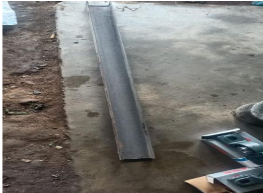
Gambar 3. 1 Besi UNP ukuran 65 mm x 40 mm x 5 mm
