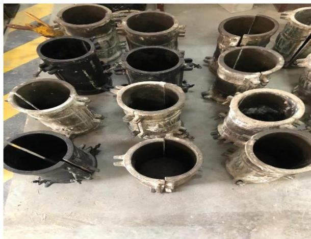
Gambar L-24: Bekisting silinder.
