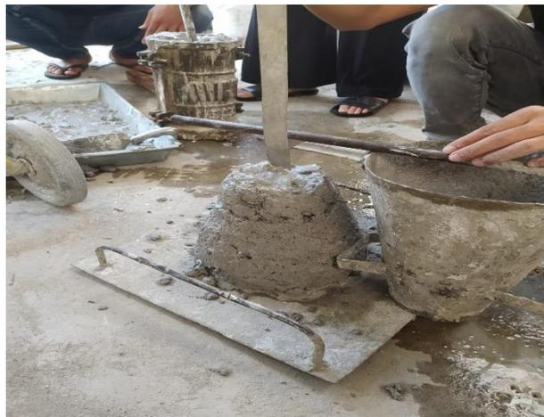
Gambar L-23: Proses pengujian *slump test*.
