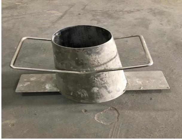
Gambar L-13: Kerucut abrams.
