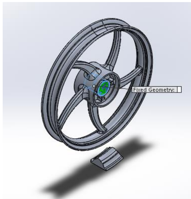
Gambar 4.12 Pemberian Fixed Geometry
