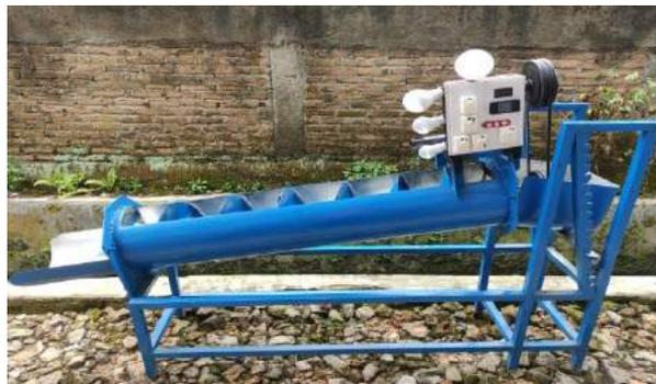
Gambar 4. Turbin Archimedes screw
