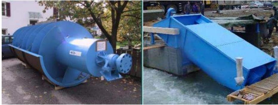
Gambar 2. Turbin Screw (a) Tipe Steel Strough dan (b) Tipe Closed Compact Installation [2](Harja et al., 2012)
