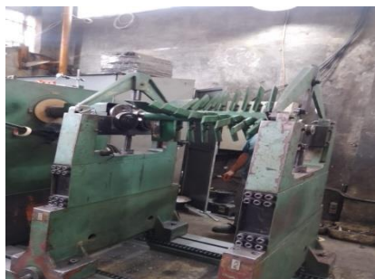
Gambar 4.1. Proses balancing mata pisau
