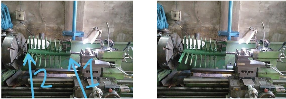
Gambar 4.2. Proses balancing mata pisau
