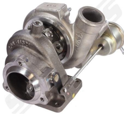
Gambar 2.17. Turbocharger Mitsubishi TD04
