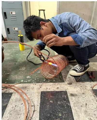
Gambar 4.14 Pengelasan Helical- Coil
