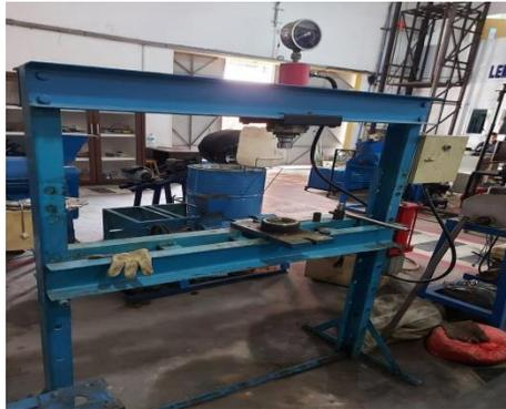
Gambar 3.9 Mesin *Press Hydraulik*
