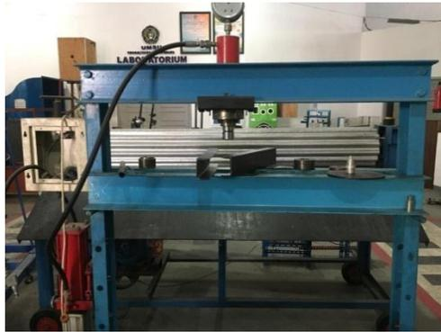
Gambar 3.1 Mesin Press Hidraulik
