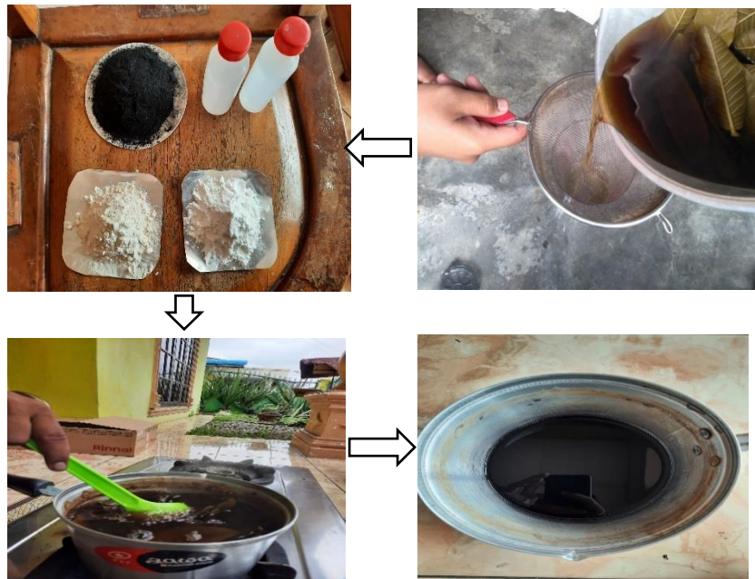
Gambar 3.2 Proses pembuatan tinta ITS Back To Nature
