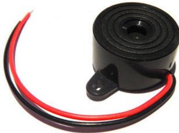
Gambar 2.14. Buzzer (Fitriandi et al. 2016)
