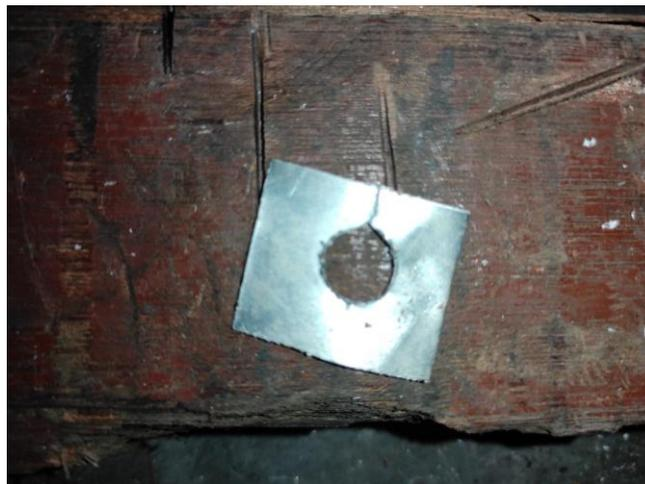
Gambar 3.2 Sirip Kondensor
