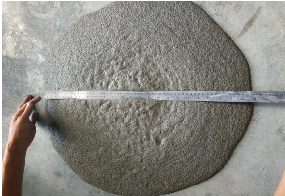
Gambar 3.33: Pengukuran Nilai Slump Flow .
