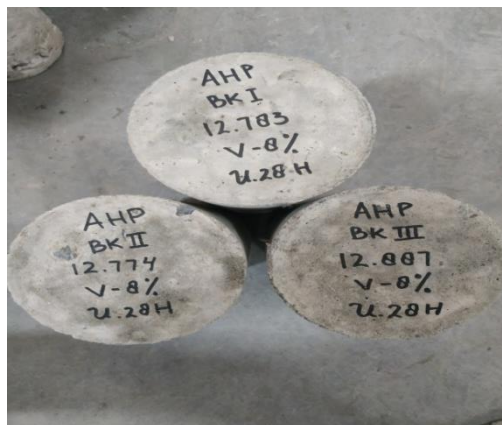
Lampiran 35: Beton V-8%.
