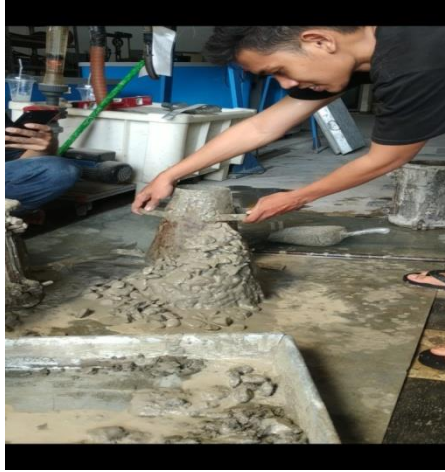
Lampiran 28: Proses pengujian slump test .
