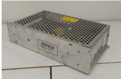
Gambar 3. 13 Power Supply 20V 10A
