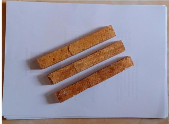
Gambar 4.2 Hasil Pengujian Spesimen *Three Point Bending* 90% resin :10% serat
