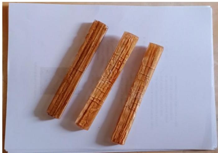
Gambar 4.4 Hasil pengujian spesimen *Three Point Bending* 80% resin : 20% serat
