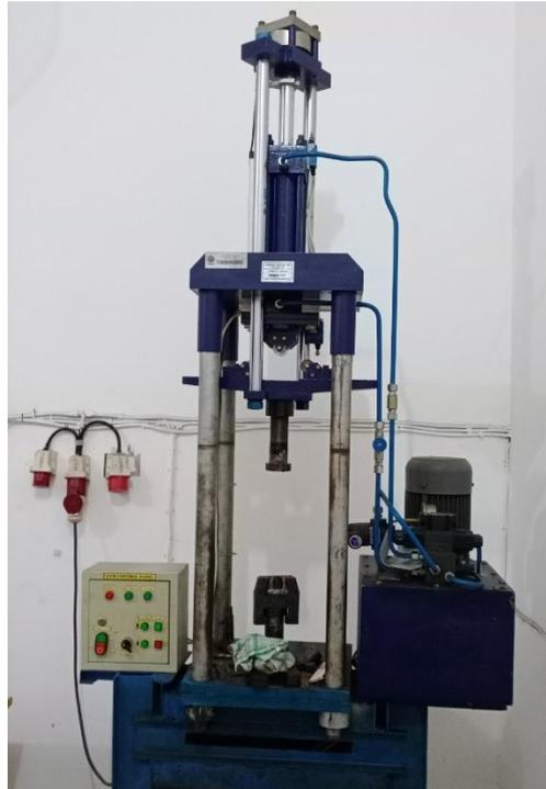
Gambar 2.11 alat uji *Three Point Bending*
