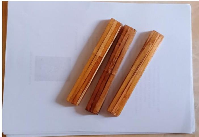
Gambar 4.3 Hasil Pengujian Spesimen *Three Point Bending* 85% resin :15% serat
