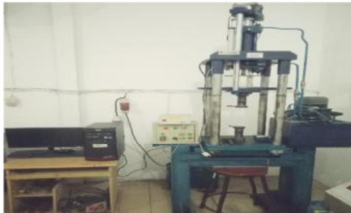
Gambar 3.1. Alat Uji Three Point Bending
