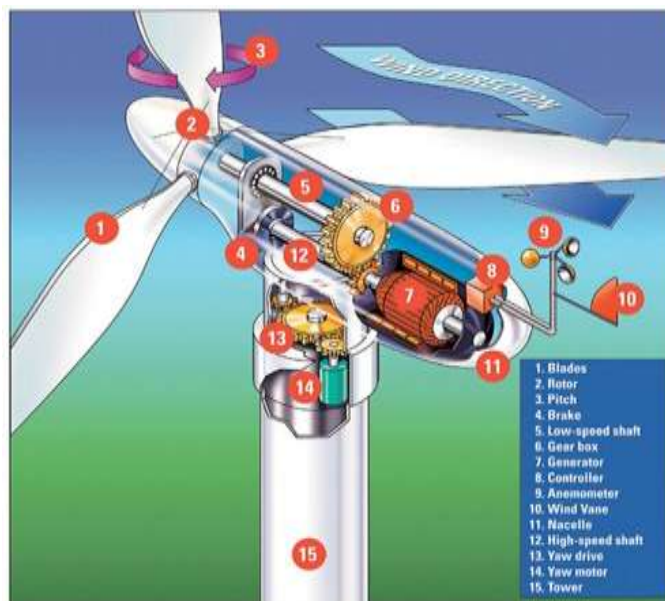
Gambar 2. 2 Bagian-Bagian Turbin Angin
