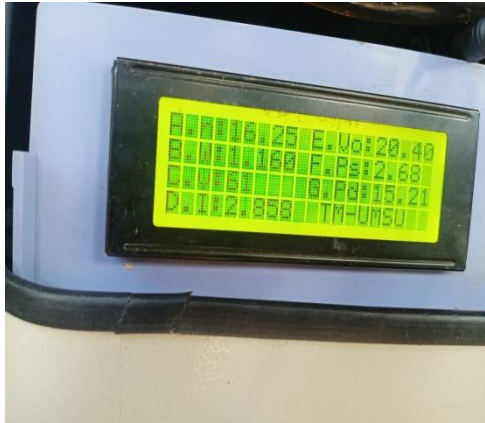
Gambar monitor pengukuran torsi, flow meter, arus, suction, discharge
