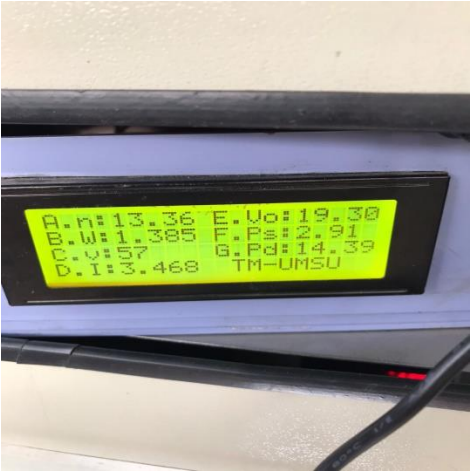
Gambar monitor pengukuran torsi, flow meter, arus, suction, discharge
