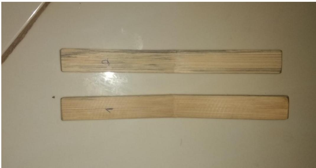
Gambar 4.4 Spesimen hasil pengujian *Three Point Bending*
