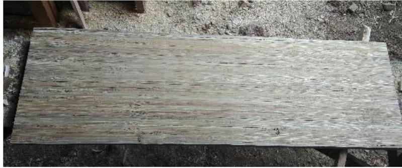
Gambar 3.28 Papan bambu laminasi ketebalan 2 cm
