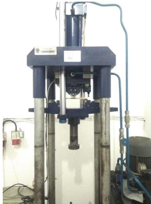
Gambar. 3.30 Alat Uji Three Point Bending
