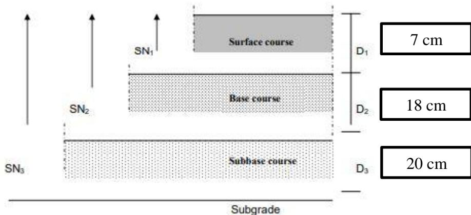
Gambar 4.6: Detail Perkerasan Metode AASHTO 1993
