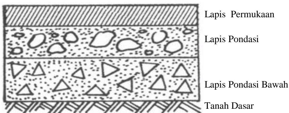
Gambar 2.1: Lapisan Konstruksi Perkerasan Lentur (Sukirman, 2010)
