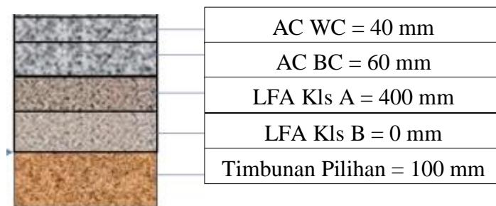
Gambar 4.2: Detail Perkerasan Metode Bina Marga 2017
